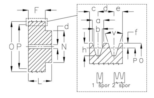
$\begin{array}{lll} d & = 10 \\ F & = 44 \\ L & = 55 \\ N & = 50 \\ Number of ribs = 2 \\ O & = 97.0 \\ P & = 90 \\ Type & = B \end{array}$
